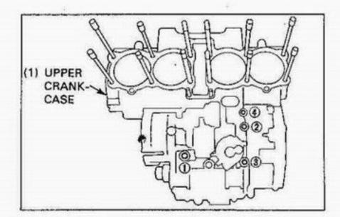
Apply a sealant to the countershaft bearing cover and clutch cover mating surfaces as shown.
