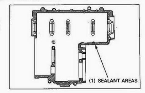
Install the crankcase bolts and sealing washers.
