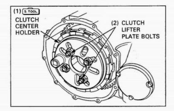
Hold the clutch center holder and torque the clutch center lock nut as shown.
