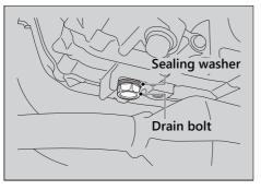
**6.** Install a new sealing washer onto the drain bolt. Tighten the drain bolt.
