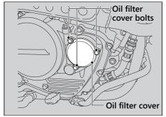
Replace the O-ring and apply a thin coat of engine oil to the new O-ring before installing it. **8.** Position the spring against the engine crankcase and install the new oil filter with the OUT-SIDE mark facing out.
