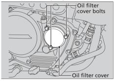
7. Replace the O-ring and apply a thin coat of engine oil to the new O-ring before installing it.
