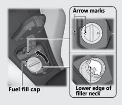
Do not fill with fuel above the lower edge of the filler neck.
