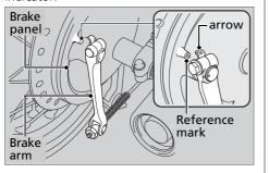
When the brake is applied, an arrow attached to the brake arm moves toward a reference mark on the brake panel. If the arrow aligns with the reference mark on full application of the brake, the brake shoes must be replaced.
