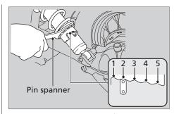
Attempting to adjust directly from 1 to 5 or 5 to 1 may damage the shock absorber.
