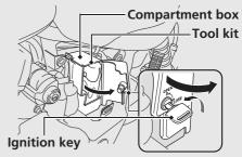
► Insert the ignition key and turn it counterclockwise to unlock.
