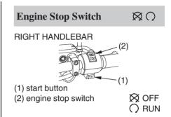
The engine stop switch (2) is used to stop the engine in an emergency. To operate, push the switch to the OFF position. The switch must be in the RUN position to start the engine, and it should normally remain in the RUN position even when the engine is OFF.
