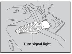
Front and rear turn signal lights use several LEDs.
