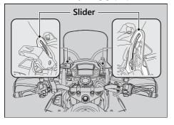
If the windscreen does not move smoothly, clean the sliders using a sponge or a soft towel with neutral detergent to remove dust.
