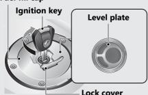
Do not fill with fuel above the level plate. **Fuel type:** Unleaded gasoline only **Recommended fuel octane number:**Pump Octane Number (PON) 91 or higher. **Tank capacity:** 5.68 US gal (21.5 L)
