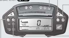
PGM-FI (Programmed Fuel Injection) malfunction indicator lamp (MIL)
