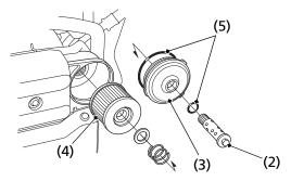
(2) oil filter bolt(3) oil filter cover
