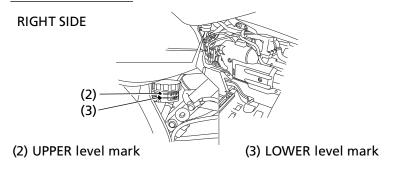
Remove the right side cover (page 71). With the ATV in an upright position, check the fluid level. It should be between the UPPER (2) and LOWER (3) level mark. If the level is at or below the LOWER level mark, check the brake pads for wear (page 148).
