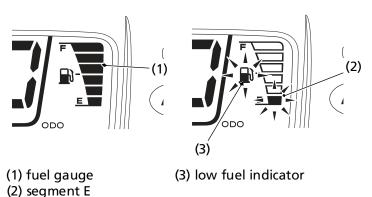
All segments will flash, when the fuel gauge function is fails. See
