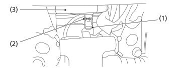
(1) drain tube (2) clip (3) air cleaner housing
