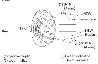
To check the condition of a tire tread, measure the groove depth (1) in the center of the tire, or check the wear indicator (2). For best performance, you should replace a tire before the tread depth at the center reaches the following limits:
