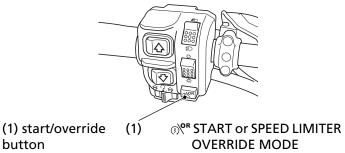
The start/override button (1) is used for starting the engine and activate the speed limiter override mode. Pushing the button in starts the engine. See *Starting Procedure*, page 86.
