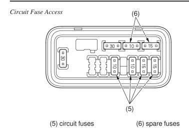
1. To check or replace a circuit fuse (5), pull the old fuse out of its retaining clips.
