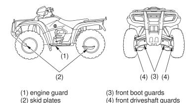
The engine guard (1) protects the engine crankcase, and the skid plates (2) protect the frame and rear final gear case.
