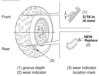
To check the condition of a tire tread, measure the groove depth (1) in the center of the tire, or check the wear indicator (2).
