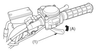
(1) throttle lever (A) to open the throttle
