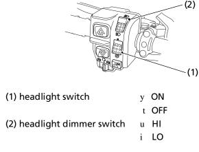
The headlight switch (1) is used to turn the headlights and assist headlight ON (y) or OFF (t). The assist headlight turns on only when the headlight dimmer switch (2) is in the HI (u) position. To operate, turn the switch to ON (y) or OFF (t).
