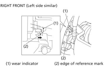
Check the wear indicator (1). If the wear indicator aligns with the edge of the reference mark (2), both pads must be replaced, see your dealer for this replacement.
