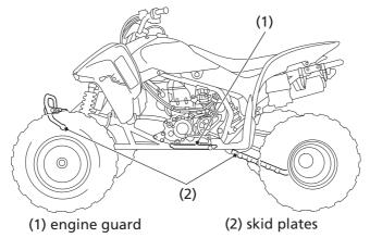
The engine guard (1) protects the engine crankcase. The skid plates (2) protect the frame/lower arm, the drive components and the rear brake. Check the guard and plates for cracks, damage or looseness at intervals shown in the Maintenance Schedule.
