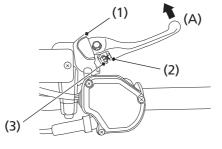
(1) brake lever cover(3) adjust bolt(2) lock nut
