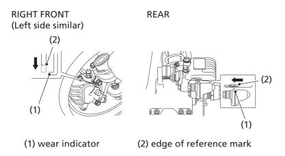
Check the wear indicator (1). If the wear indicator aligns with the edge of the reference mark (2), both pads must be replaced, see your dealer for this replacement.
