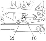
(1) transmission oil drain bolt (2) sealing washer
