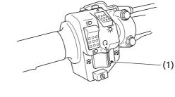
(1) engine stop switch e RUN r OFF
