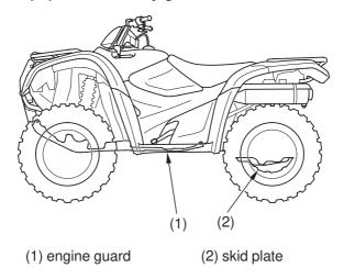
The engine guard (1) protects the frame and engine crankcase. The skid plate (2) protects the rear final gear case. Check the guard and plate for cracks, damage or looseness at intervals shown in the Maintenance Schedule.
