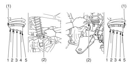
(1) spring pre-load adjuster(2) pin spanner
