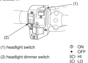
The headlight switch (1) is used to turn the headlight ON (  $\mbox{\ensuremath{\promset}\xspace}$ ) or OFF (  $\mbox{\promset}$ ). To operate, turn the switch to ON (  $\mbox{\ensuremath{\promset}\xspace}$ ) or OFF (  $\mbox{\promset}$ ).
