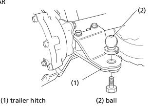
The trailer hitch (1) is located on the rear axle housing. To use the hitch, you'll need a proper size ball (2) as specified by the trailer manufacturer.
