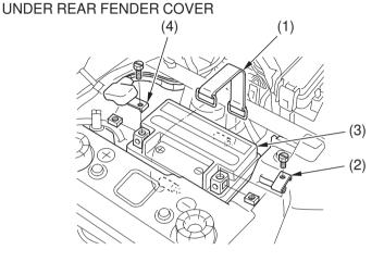
(1) rubber band(3) battery(2) negative (-) terminal lead(4) positive (+) terminal lead
