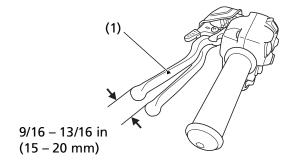
(1) rear brake lever/parking brake lever
