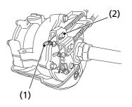
(1) brake lever adjusting nut
