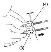
(2) brake pedal adjusting nut(3) brake arm pin
