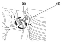
(5) lower adjusting nut(6) lower lock nut
