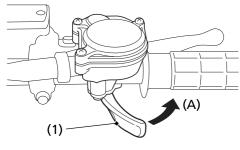
(1) throttle lever(A) to open the throttle
