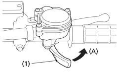
(1) throttle lever(A) to open the throttle
