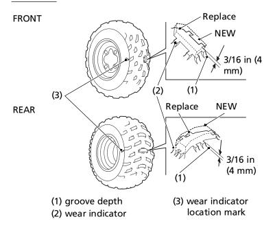
To check the condition of a tire tread, measure the groove depth (1) in the center of the tire, or check the wear indicator (2). For best performance, you should replace a tire before the tread depth at the center reaches the following limits:
