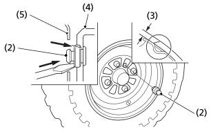
(2) inspection hole plug (3) lining thickness (4) front brake drum (5) front wheel rim
