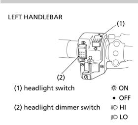
The headlight switch (1) is used to turn the headlight ON  $(\clubsuit)$  or OFF (•). To operate, turn the switch to ON  $(\clubsuit)$  or OFF (•).
