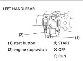
The start button (1) is used for starting the engine. Pushing the button in starts the engine. See *Starting Procedure*, page 49.
