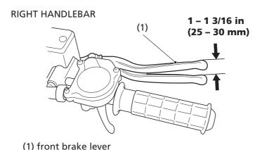
1. Measure the distance the brake lever moves before the brakes start to take hold. Freeplay, measured at the tip of the front brake lever (1)
