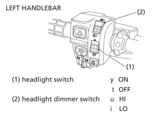
The headlight switch (1) is used to turn the headlight ON (y ) or OFF (t). To operate, turn the switch to ON (y ) or OFF (t).
