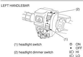
The headlight switch (1) is used to turn the headlight ON ( $\mbox{\ensuremath{\@psi}}$ ) or OFF ( $\mbox{\ensuremath{\@psi}}$ ). To operate, turn the switch to ON ( $\mbox{\ensuremath{\@psi}}$ ) or OFF ( $\mbox{\ensuremath{\@psi}}$ ).
