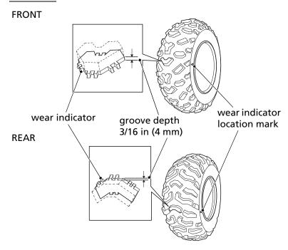
To check the condition of a tire tread, measure the groove depth in the center of the tire, or check the wear indicator.
